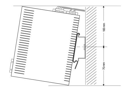
• Insert the module that you are installing into the profile rail at an angle of about 45 degrees from the top and rotate the module into place until it clicks into the profile rail with an audible click.
