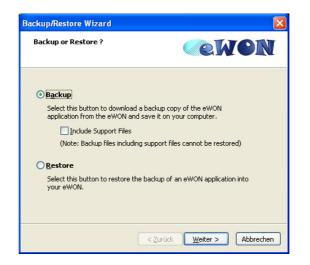
Backup Open the dialog window with clicking to "Backup/restore application". Select "Backup". Even if you want to forward the backup to the VIPA support the files relevant to the support should also be saved. Here activate the option "Include support files". Click to [Continue >].
