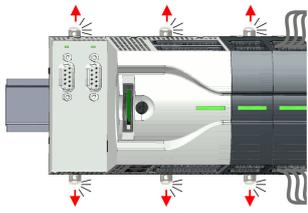
1. ➤ Remove the modules that are connected to the module to be replaced by pulling their release levers outwards until these engage audible ...
